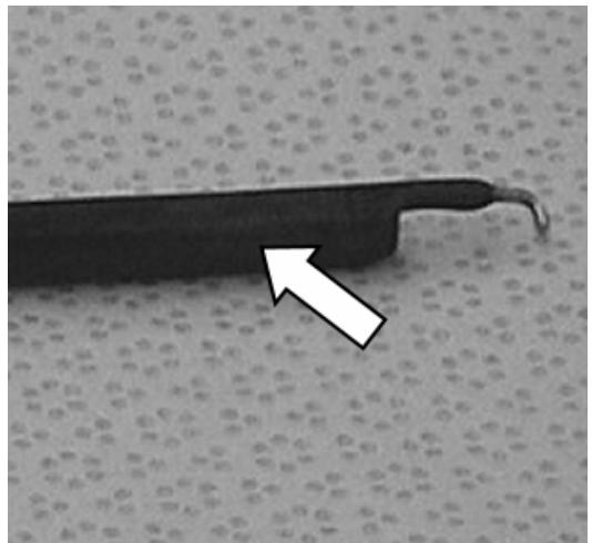
Microscopic insulation defect on a hook (arrow).
