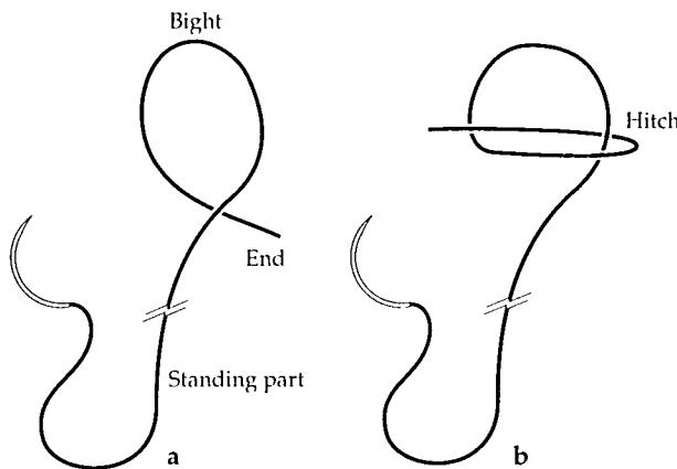
Figure 1. a) Knot-tying terms. b) A simple hitch.
