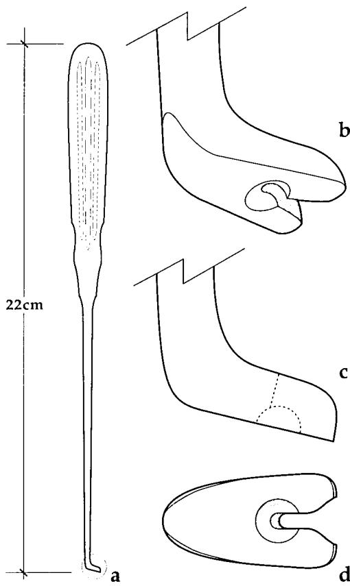
**Figure 4.** a) The forked knot pusher. b) Angled view of the base showing the V-shaped groove and countersunk area. c) Side views with the broken lines showing the countersunk area and the V-shaped groove. d) View of undersurface of the base.
